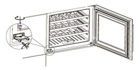
1. Put the wine cooler into the cabinet, then adjust the wine cooler to make it steady. Open the door, take
